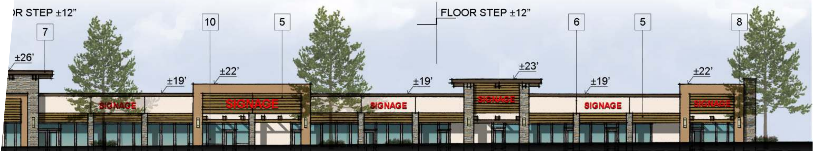
SHOP TENANT- PARTIAL SOUTH EAST ELEVATION SCALE: 1/16"=1'-0"
