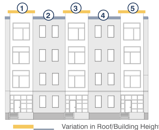
FIGURE 3.13: REPEATED ROOF TYPES: FLAT ROOF "SAWTOOTH"
