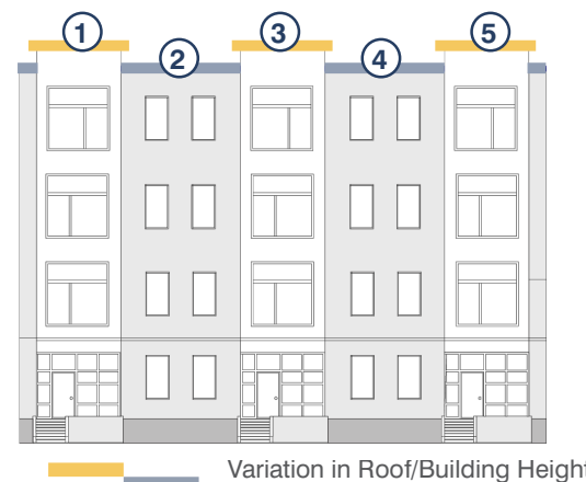
FIGURE 3.13: REPEATED ROOF TYPES: FLAT ROOF "SAWTOOTH"
